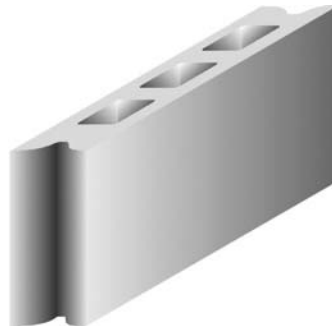
CONCRETE BLOCK 40 x 20 x 9 WEIGHT: 10kg CONSUMPTION: 12.5 pcs/m 2
